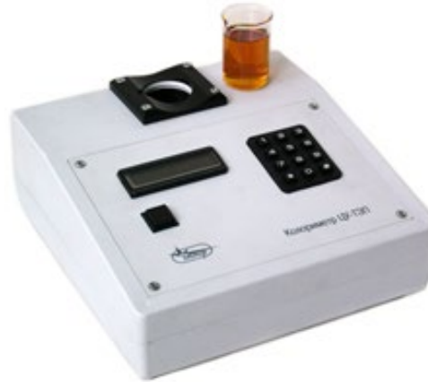
Automatic color analyzer TSU TEP-I-3;4 of vegetable oils (sunflower, rapeseed, etc.) in accordance with domestic and international standards ISO 15305, DSTU 4568: 2006, etc.
