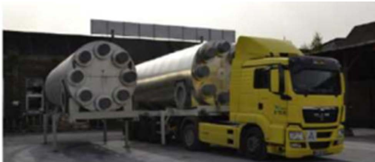
Photos of the M-TES prototype developed by the Fraunhofer UMSICHT Institute: a) External heat exchanger of the container, b) Transportation of the M-TES container**
