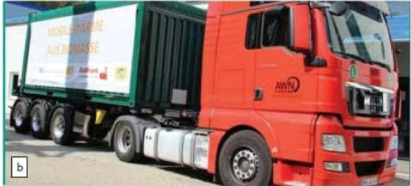
Photos of the M-TES prototype developed by the Fraunhofer UMSICHT Institute: a) External heat exchanger of the container, b) Transportation of the M-TES container**
