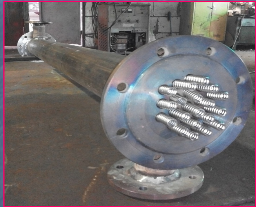
Heat exchanger ТО-75
