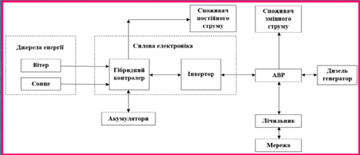
The block diagram of the electric power supply of the passive house of "0 energy" type
